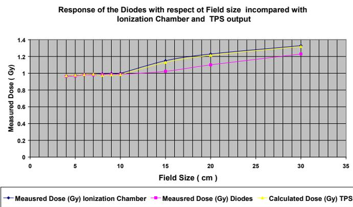
Fig 2: Response of the Diodes with respect to field size in compared with ionization chamber and TPS output.
