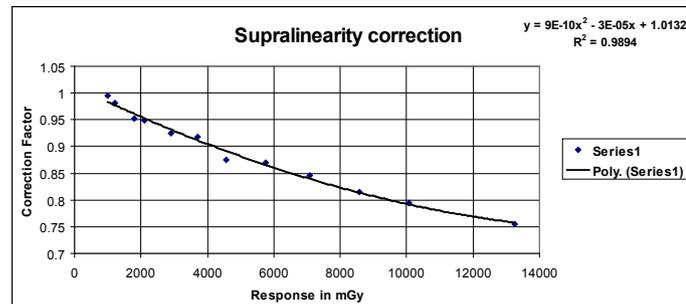
Fig 9: Supralinearity correction for TLD patches as function in different doses in cGy.
