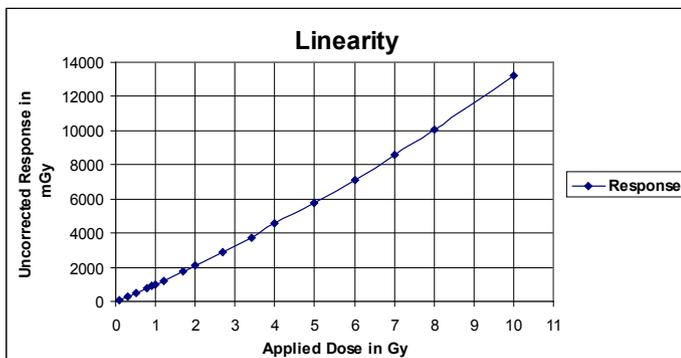
Fig 8: Linearity for TLD patches as function in different doses.
