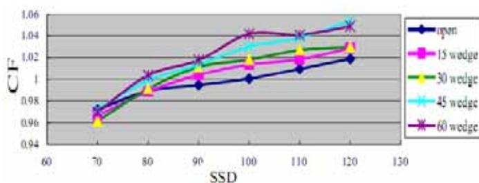
Fig 5: Diode correction factors as a function of the SSD for entrance measurements; (15MV photon). All data in this figure are for field size 10x10cm<sup>2</sup>.
