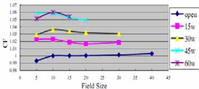
Fig 3: Correction factor of 6MV – diode of as a function of the field size, FS for Open field and different Wedge Angles, for entrance measurements. All data in this figure are for SSD 100 cm and ratio to ionization as standard (for standard Field size 10 X10 cm<sup>2</sup>). (Max Sq.field size for W 60 is 15 cm).
