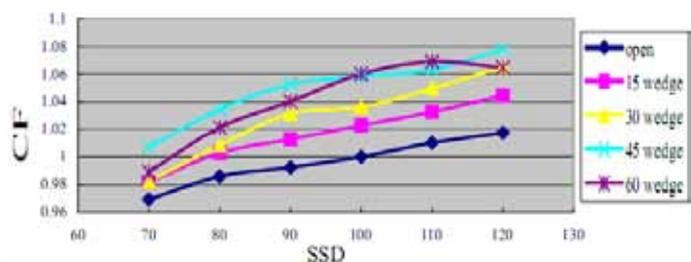
Fig 4: Diode correction factors as a function of the SSD for entrance measurements. All data in this figure are for field size 10x10 cm<sup>2</sup> (6MV photon).
