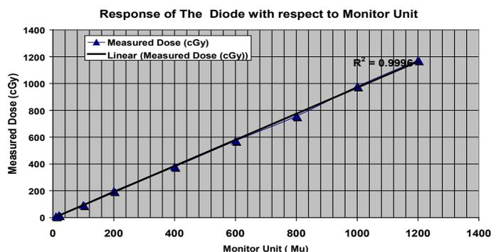
Fig 1: Response of the Diode with respect to Monitor Unit (Mu).
